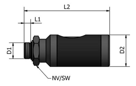
D1 = G 1/4 D2 (mm) = 26 L1 (mm) = 6.5 L2 (mm) = 70 SW (mm) = 21 Weight (g) = 144
